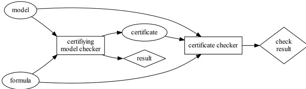
FIGURE 1.2. Certified model checking workflow.
