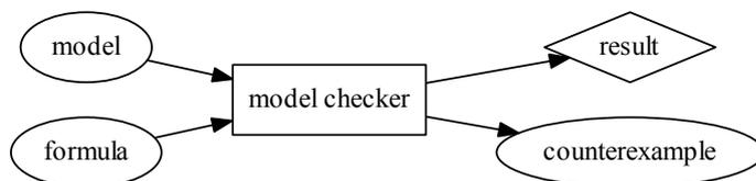
FIGURE 1.1. Standard model checking workflow.
